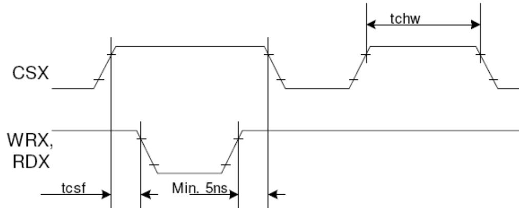
*Note: Logic high and low levels are specified as 30% and 70% of VDDI for Input signals.*
